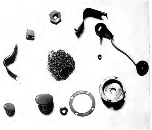
FIG. 26.—PARTS OF TRANSMITTER CAPSULE.
